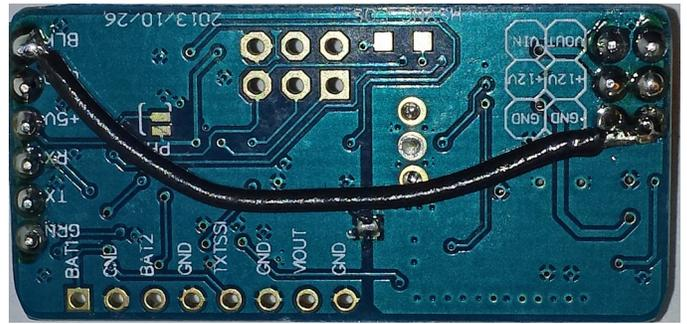
This jumper will prevent burning out MinumOSD if to much Current tries to flow through it's small ground trace
