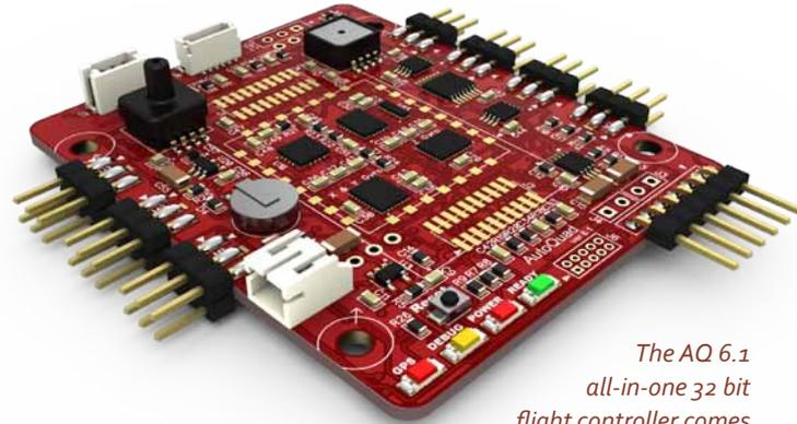
*The AQ 6.1 all-in-one 32 bit flight controller comes with a complete set of precision analog sensors and accurate UBlox LEA GPS module*
